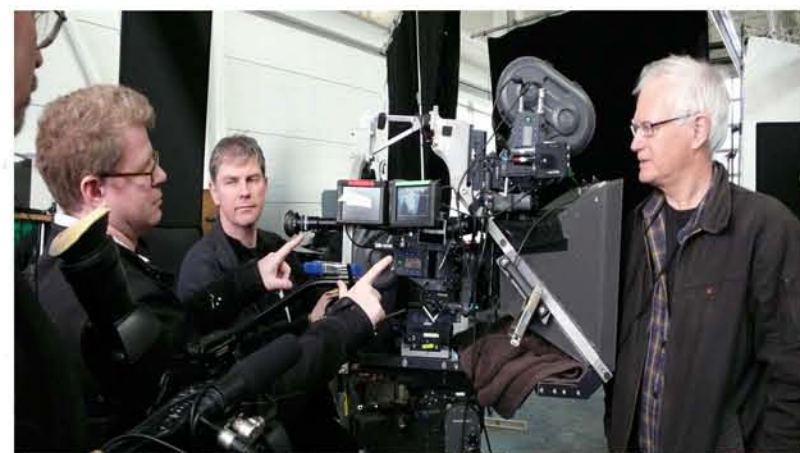
James Stewart of Geneva Film uses two digital cameras mounted on top of one another with a mirror rig to shoot identical images, one representing the left eye, the other the right
